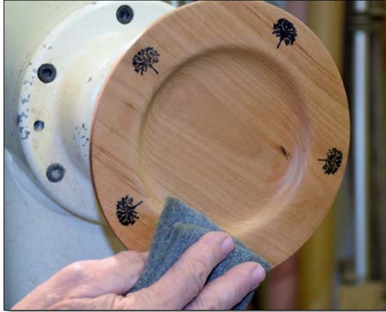
Photo 8: Lightly rubbing the plate to remove dust nibs after a coat of varnish has dried.
