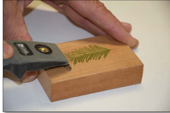
Photo 9: Using a paint scraper to remove an embossed design.
