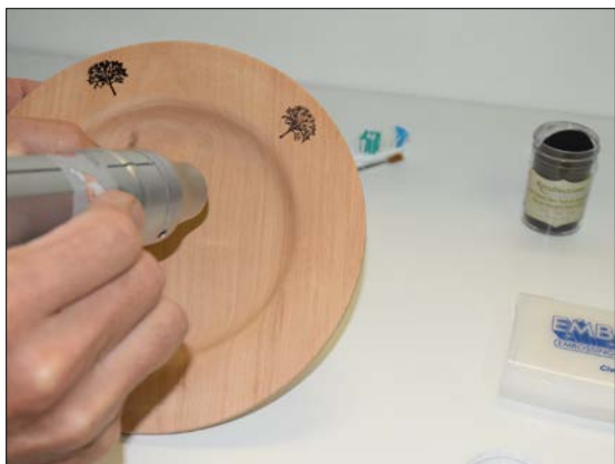
Photo 6: Heating the powder to melt and bond it to the wood.
