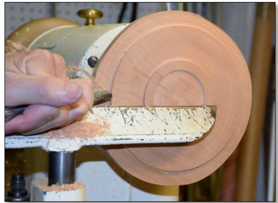
Photo 1: Preparing the base of a cherry plate with a recess to mount on a 4-jaw chuck.
