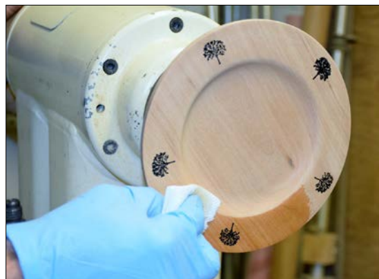
Photo 7: Applying varnish to the plate.
